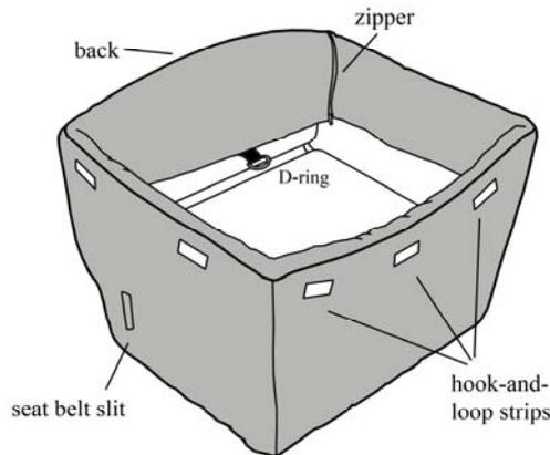
The underside of the Inner Fabric Liner also has two small tags marked “X” and “Z”. Insert the inner liner into the seat portion of the plastic frame so the “X” and “Z” seams on the inner liner align with the “X” and “Z” seams on the outer shell. Fit the upper edge of the fabric liner over the rear wall of the plastic frame and fasten the loop tape pieces on the inner liner with the hook tape pieces on the outer shell.
