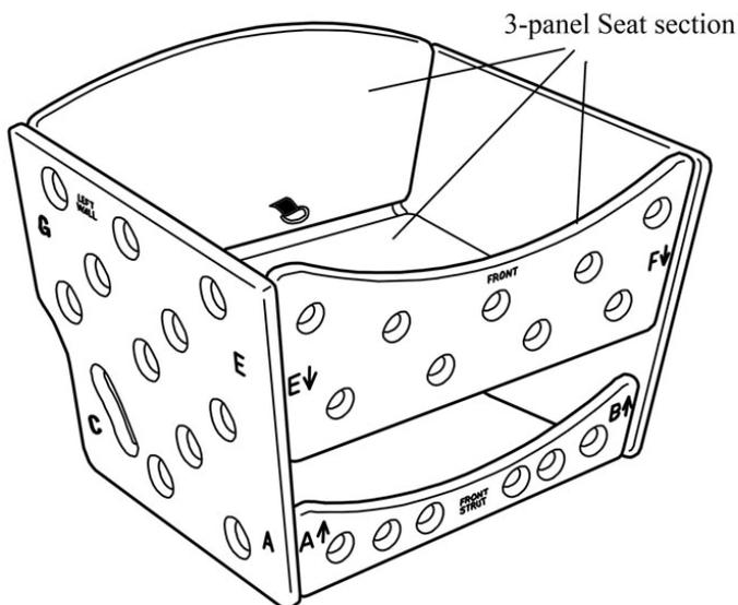
The Seat section is a three-panel piece that was folded in a “Z” shape in the package. Before connecting to the Left and Right Wall sections, fold the Seat section into a “U” shape with the smooth sides facing “in”. Insert double-tab E on the front panel of the Seat section into slot E on the Left Wall and slide to lock. Repeat for tab G then repeat for tabs F and H into the corresponding slots on the Right Wall.
