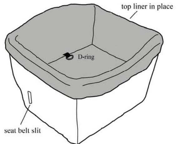
To install in vehicle, place the booster on the vehicle seat and pass the seat belt through the holes in the fabric and plastic frame on one side of the booster.
