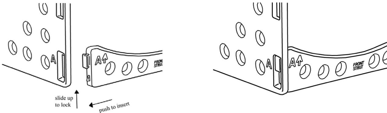
Repeat this procedure to lock tab B on Front Strut into slot B on Right Wall, and to lock tabs C and D on Rear Strut into slots C and D on the Left and Right Wall sections.
