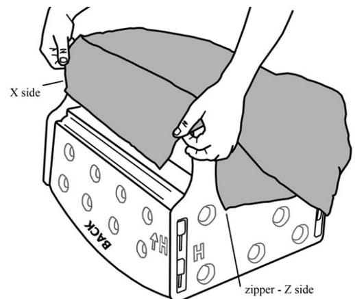
Place the assembled plastic frame upside-down on a clean surface. The Outer Fabric Shell has a zipper and small tags marked “Z” (next to zipper) and “X” (on opposite seam). With zipper in the fully open position, slide the fabric shell over the plastic frame so the “Z” seam aligns with the “H” corner at the back of the plastic frame and the “X” seam aligns with the “G” corner.
